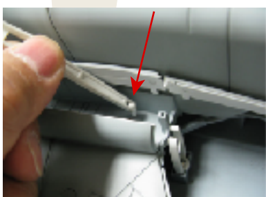
16. insert and lock locking pin for forward support arm
