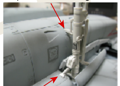
15. Lock rear and side fuselage locking arms
